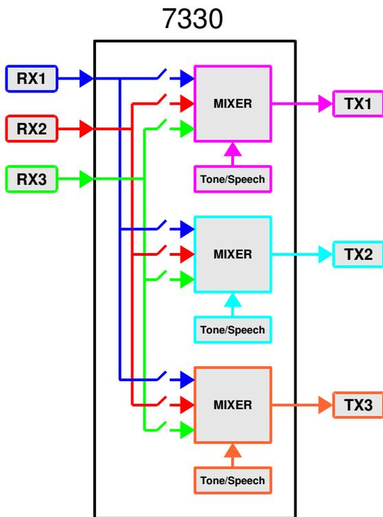
You can configure your system any way you wish by programming the nine paths that connect the three receivers to the three transmitters.
